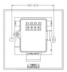
Z1, Z2: Connecting to the loop of control panel, non-polarized
